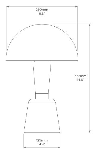
Due to the hand-crafted nature of some products, stated dimensions may have a tolerance of  $\pm \frac{1}{4}$  /6mm. If tighter tolerances are required for a specific installation, please state on your enquiry
