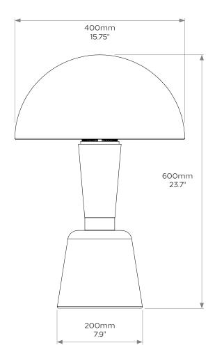
Due to the hand-crafted nature of some products, stated dimensions may have a tolerance of  $\pm \frac{1}{4}$ /6mm. If tighter tolerances are required for a specific installation, please state on your enquiry
